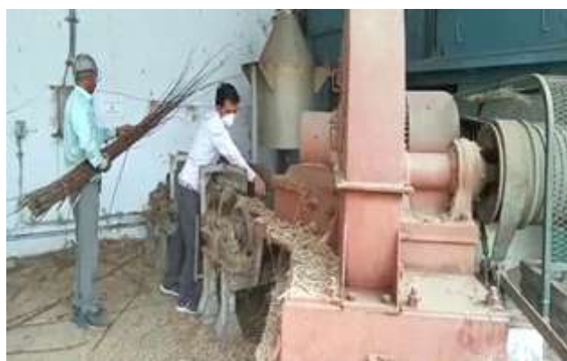
Chipping of whole jute in Disc Chipper at CPPRI Pilot Plant
