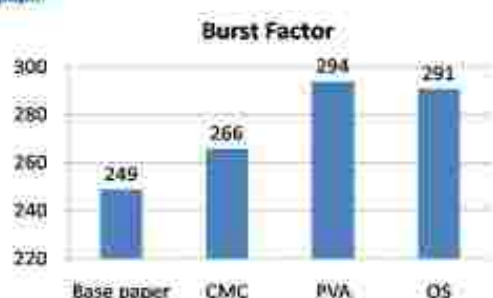
Impact of coating of different Biopolymer on Burst Factor of paper
